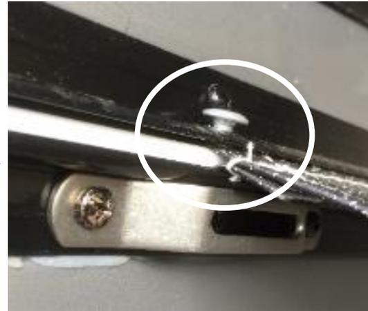
**DRILLING HOLES IN AWNING ROLLER TUBE...** mark roller tube 15mm in from the awning cloth edge and 25mm up from the groove in the roller tube, both ends. Pre-drill at mark and increase until hole size is 10mm, drag down drill to elongate the hole slightly.
