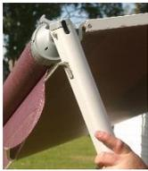
3. Disconnect awning support legs from bottom of van and swing into upright position. Adjust legs so awning groove is approx. 1905mm (6'3") from ground. For caravan applications please be sure to adjust height to clear caravan door if necessary)
